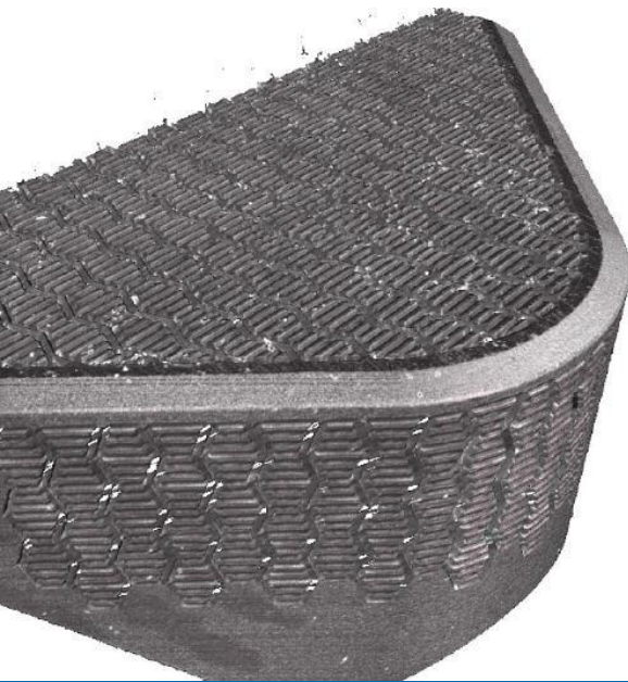
Shark skin texture produced at microlaser cell
