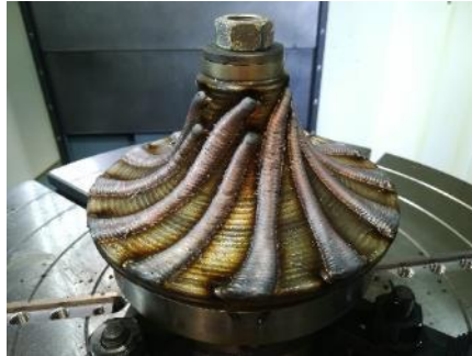
The first layer of the blade base
