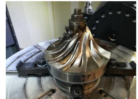
Test machining of blades
