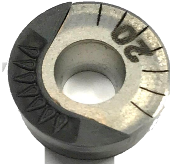
A chipbreaker in PCD tool created by laser
