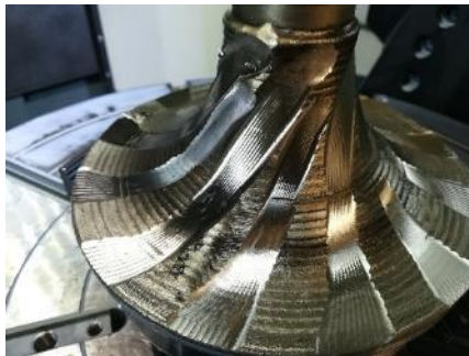
Milling bases for laying blades
