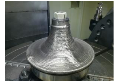
Weld base laser on the turned stock
