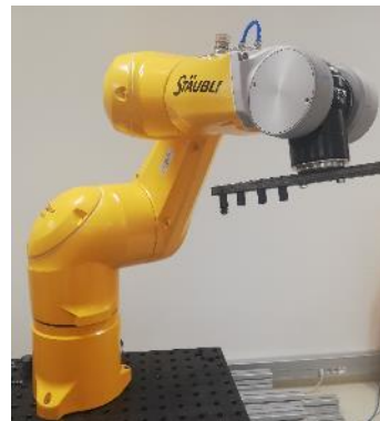
Kalibrace robotu Staubli TX2-90 tzv. metodou kružnic
